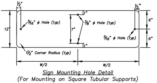
Sign Mounting Hole Detail (For Mounting on Square Tubular Supports)
