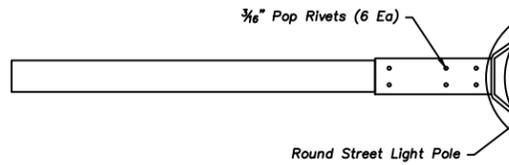
Street Name Sign Wing Bracket Detail for Round Tubular Supports
