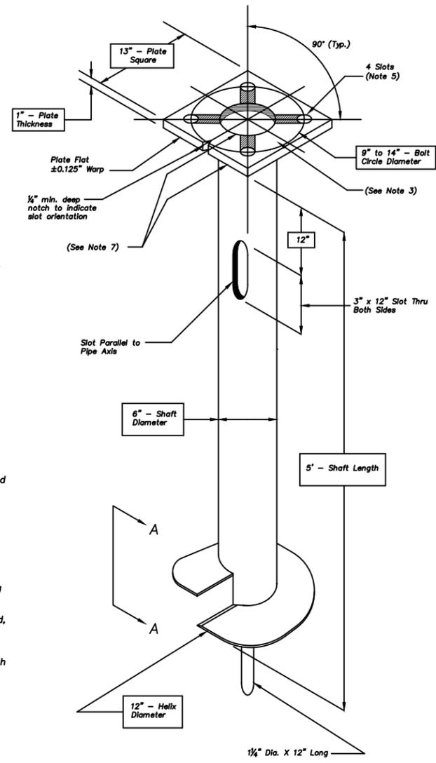
Alternate Screw-in Foundation Anchor Details
