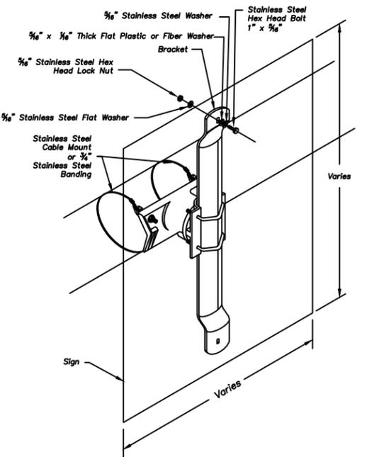
**Sign Mounting Detail (Mast Arm) (Does not apply to overhead street name signs)**
