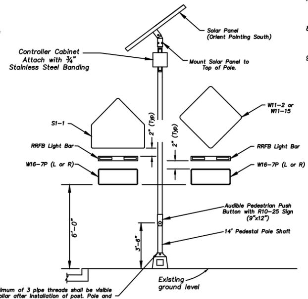
Aluminum Signal Pedestal Pole with Rectangular Rapid Flashing Beacon (RRFB)
