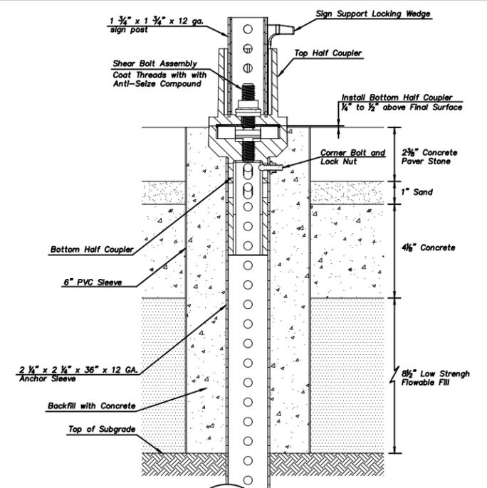
**Break-Away Sign Post Anchor Detail (Concrete Paver Stone Median/Island Mount)**
